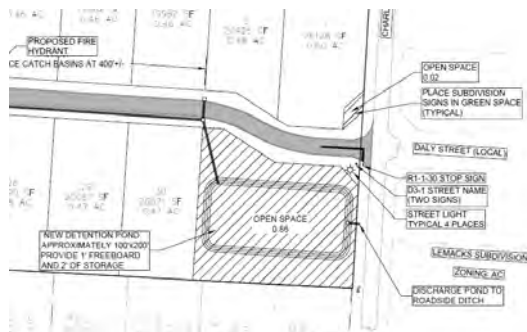
Figure 3 - Stormwater Detention Area
