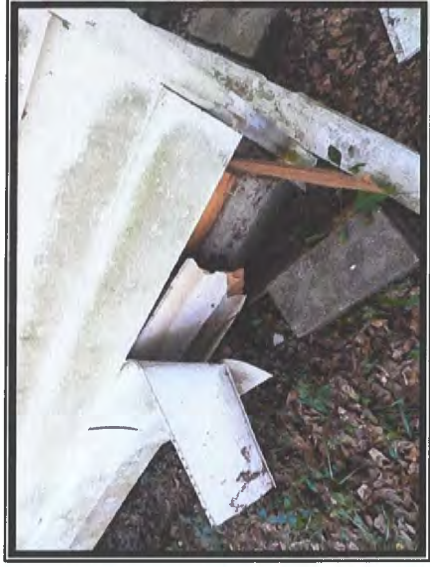
Photo #2 No Asbestos Detected in Exterior Fiberboard Wall Panels or Sheathing Board
